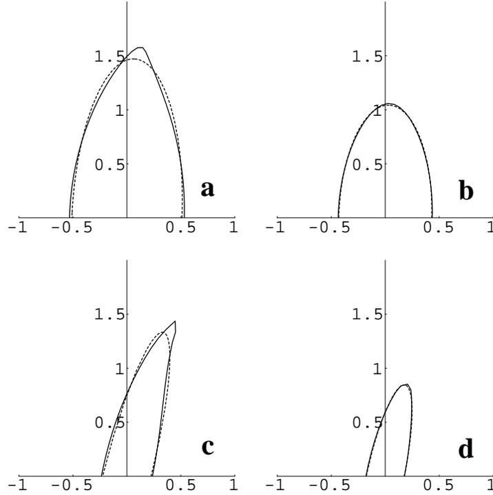
FIGURE 4. Vorticity contours (solid) and fitted ellipses (dotted) for experiment 2. Upper row:  $t = 57$ , and (a)  $\omega = 0.25\omega_0$  (contour 6), (b)  $\omega = 0.55\omega_0$  (contour 12). Lower row:  $t = 63$ , and (c)  $\omega = 0.7\omega_0$  (contour 15), (d)  $\omega = 0.85\omega_0$  (contour 18).
