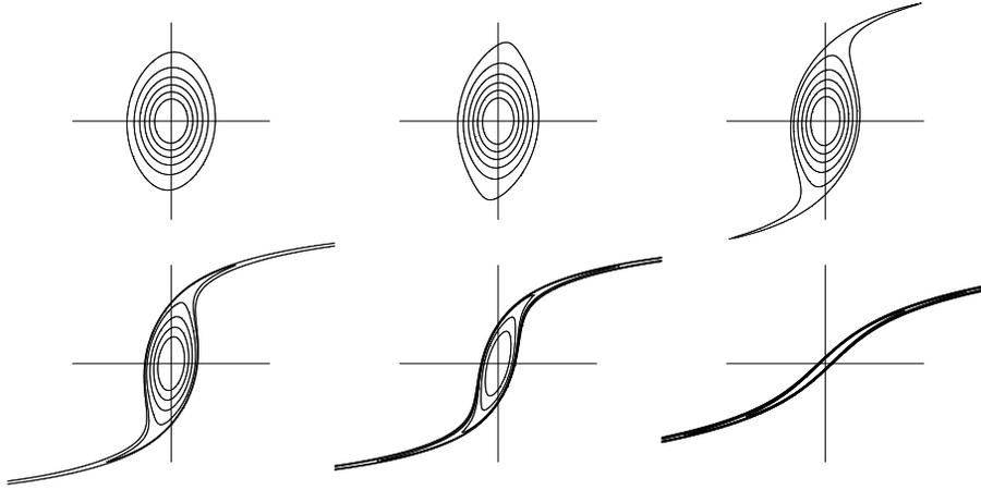
FIGURE 1. Vorticity charts at times  $t = 26, 31, 36, 41, 46, 51$  from left to right and from top to bottom for experiment 1, conducted using the PS method with a small viscosity. The vortex is initially Gaussian and is subjected to a linearly growing adverse shear. The contour interval is 0.8.
