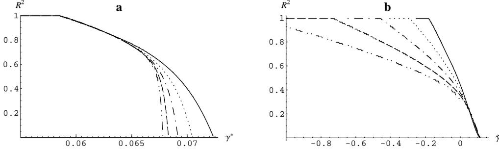
FIGURE 11. (a) Erosion curves for the EM+C defined as in figure 10.  $---$ ,  $\tau = 1250$ ;  $\cdots$ ,  $\tau = 2500$ ;  $-\cdot-\cdot-$ ,  $\tau = 5000$ ;  $---$ ,  $\tau = 10000$ ;  $-\cdot\cdot\cdot$ ,  $\tau = 20000$ . (b) The same after rescaling  $\gamma^*$  into  $\tilde{\gamma} = (\gamma^* - \gamma_c)(\tau\omega_0)^{2/3}$ .
