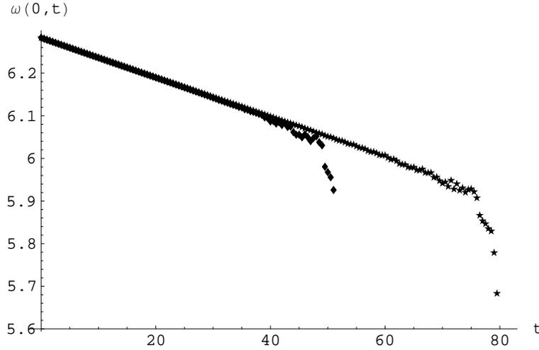
FIGURE 16. Evolution of the maximum vorticity at the centre of the vortex.  $\blacklozenge$ , experiment 1;  $\star$ , same as experiment 1 but with half the strain growth rate. Solid line, curve predicted by (6.3).
