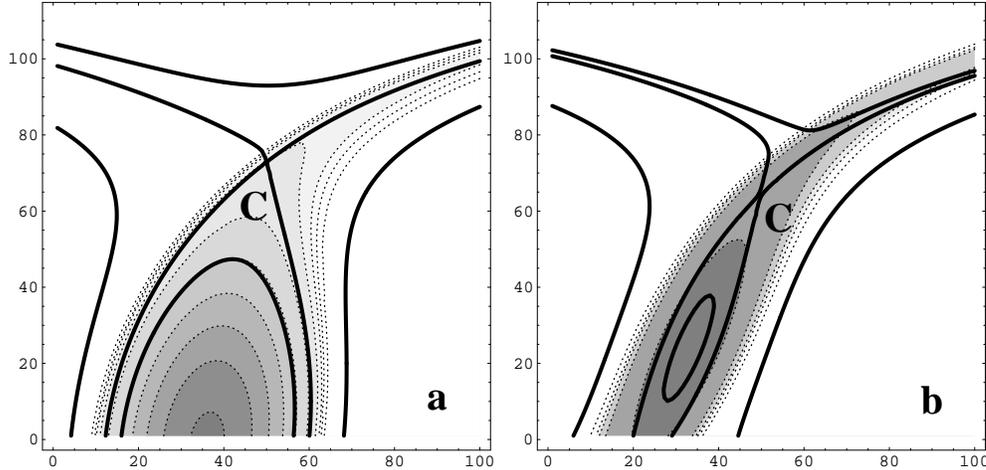
FIGURE 6. (a) Enlargement of the vorticity chart at  $t = 42$  for experiment 1. Thick solid line: the separatrices, crossing at the critical point  $C$ , and other selected streamlines. Dotted line: vorticity contours with contour interval  $0.1\omega_0$ . Axis labels are in units of the collocation grid. (b) Same but at  $t = 48$  and with a contour interval  $0.2\omega_0$ . The enlarged window has the same size in (a) and (b) but has a different centre.
