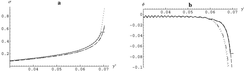
FIGURE 9. (a) Evolution of the eccentricity as a function of the strain for  $\tau = 2500$ . For CS:  $-\cdot-$ ,  $\sigma(0)$ ;  $\cdots$ ,  $\sigma(0.6)$ . For EM+C:  $---$ ,  $\sigma(0)$ ;  $---$ ,  $\sigma(0.6)$ . (b) Evolution of the orientation  $\phi$  for the same case. The EM+C curves for the radius  $r = 0.6$  level off after the elimination of this contour.
