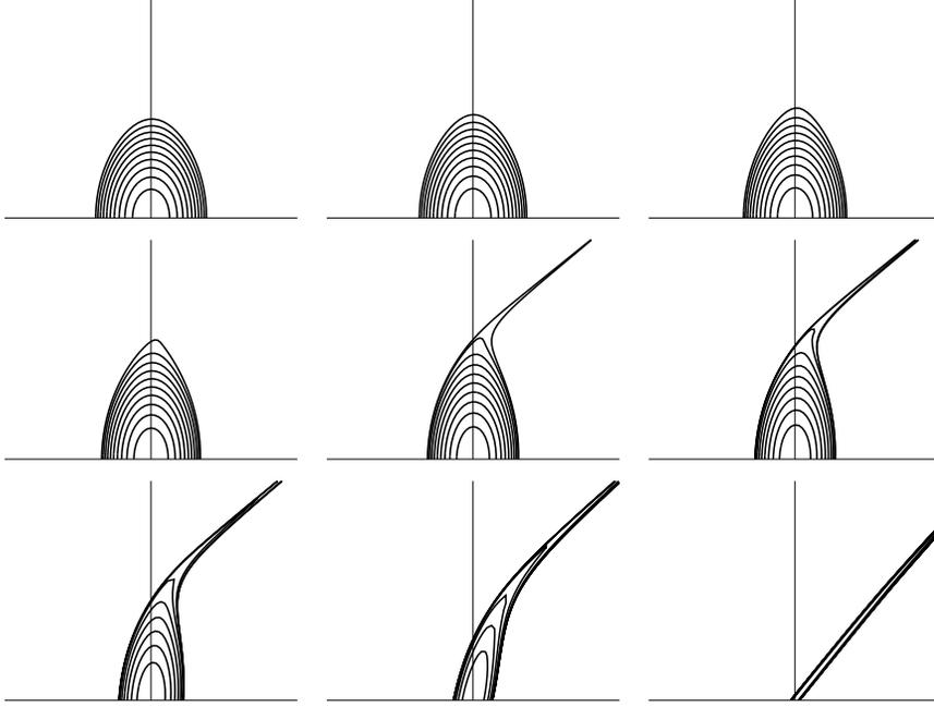
FIGURE 3. Vorticity charts at times  $t = 42, 45, 48, 51, 54, 57, 60, 63, 66$  from left to right and top to bottom for experiment 2, conducted using the CS method. The vortex is initially parabolic and is subjected to a linearly growing pure shear. All 20 contours are plotted but several contours at the vortex edge have become indistinguishable as a result of stripping.
