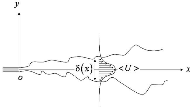
**Fig.1** – Turbulent jet
