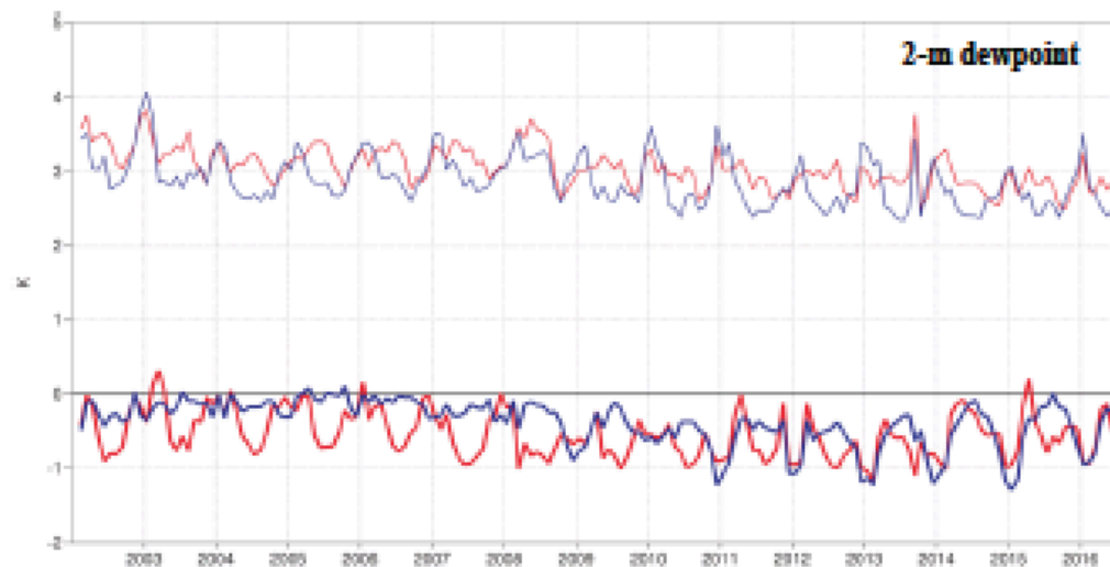
Figure 20: Verification of 2 m dew point forecasts against European SYNOP data on the Global Telecommunication System (GTS) for 60-hour (night-time) and 72-hour (daytime) forecasts. Lower pair of curves shows bias, upper curves show standard deviation of error.
