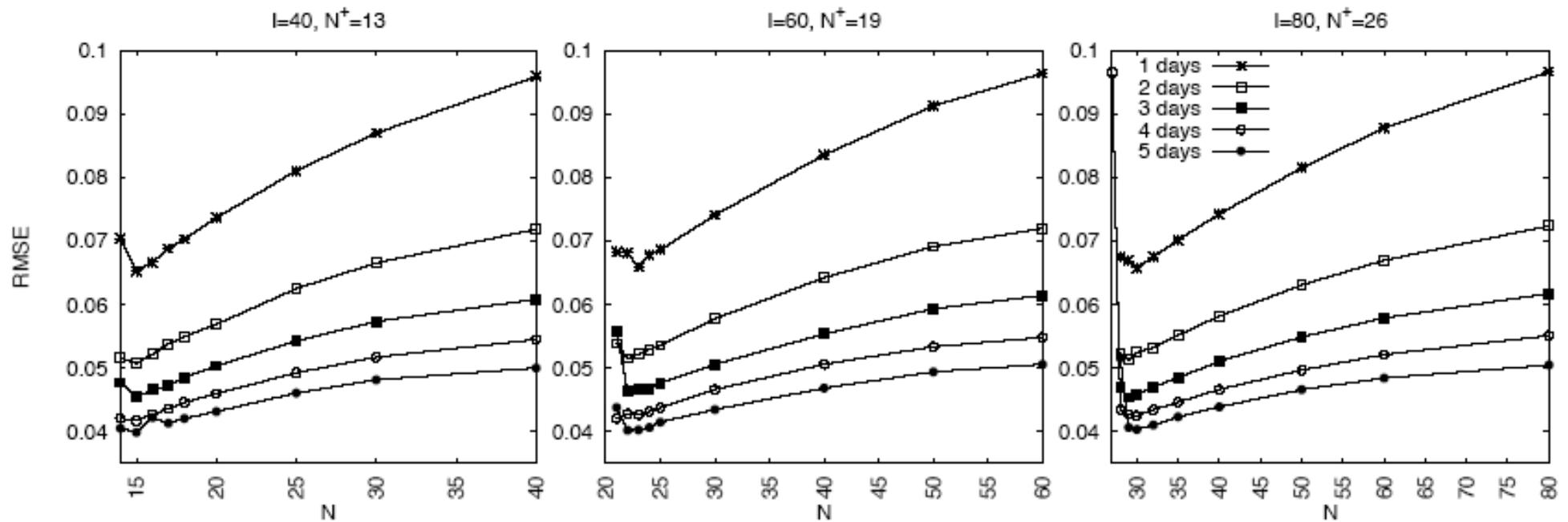
Figure 1. Time average RMS analysis error at  $t = \tau$  as a function of the subspace dimension  $N$  for three model configurations:  $I=40, 60, 80$ . Different curves in the same panel refer to different assimilation windows from 1 to 5 days. The observation error standard deviation is  $\sigma_o = 0.2$ .
