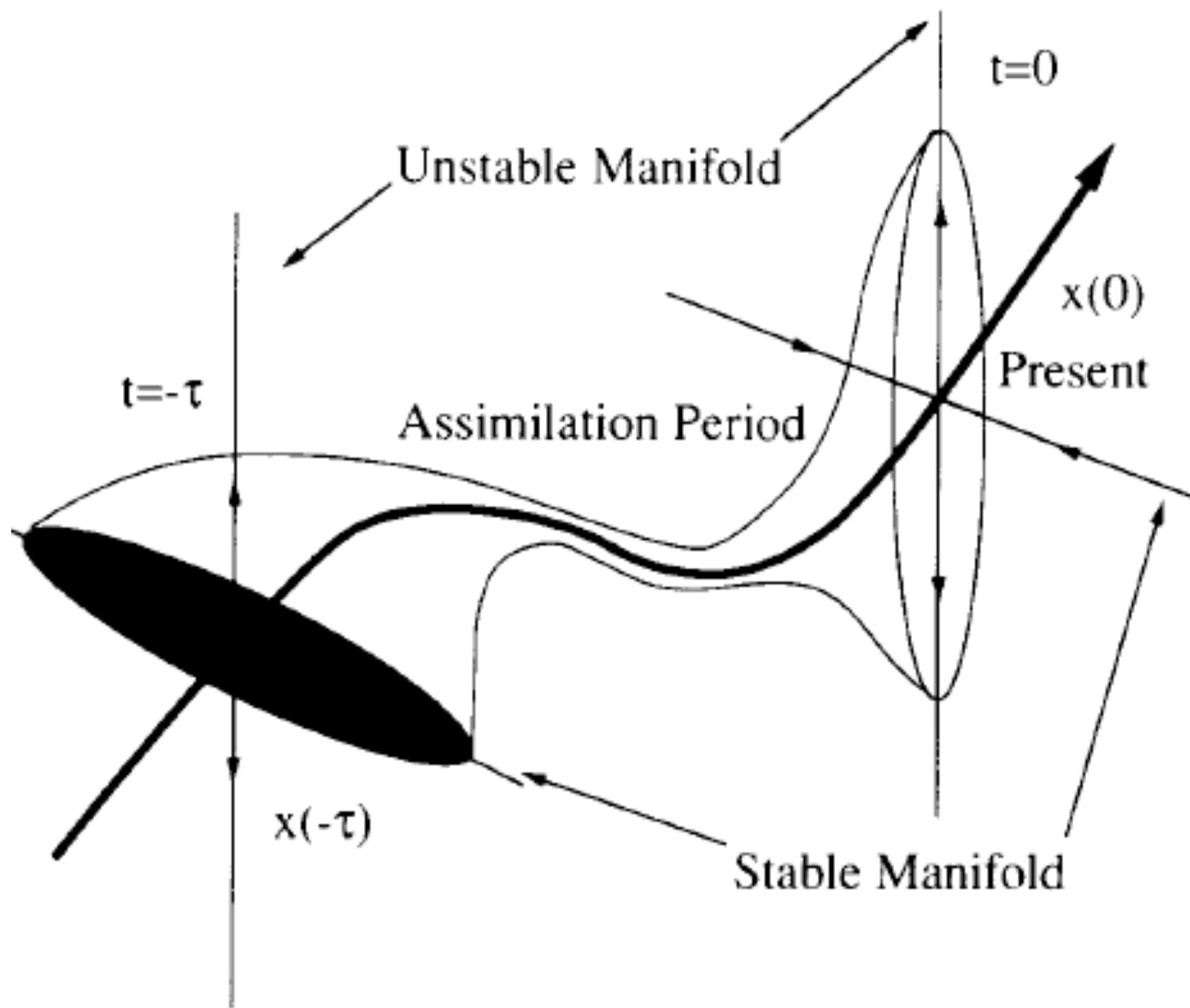
Gurumoorthy *et al.* (2017a, 2017b) have shown that in the linear perfect model case, the error covariance matrix of the Kalman filter converges to the neutral-unstable subspace of the system (space spanned by the non-negative Lyapunov exponents of the system)
