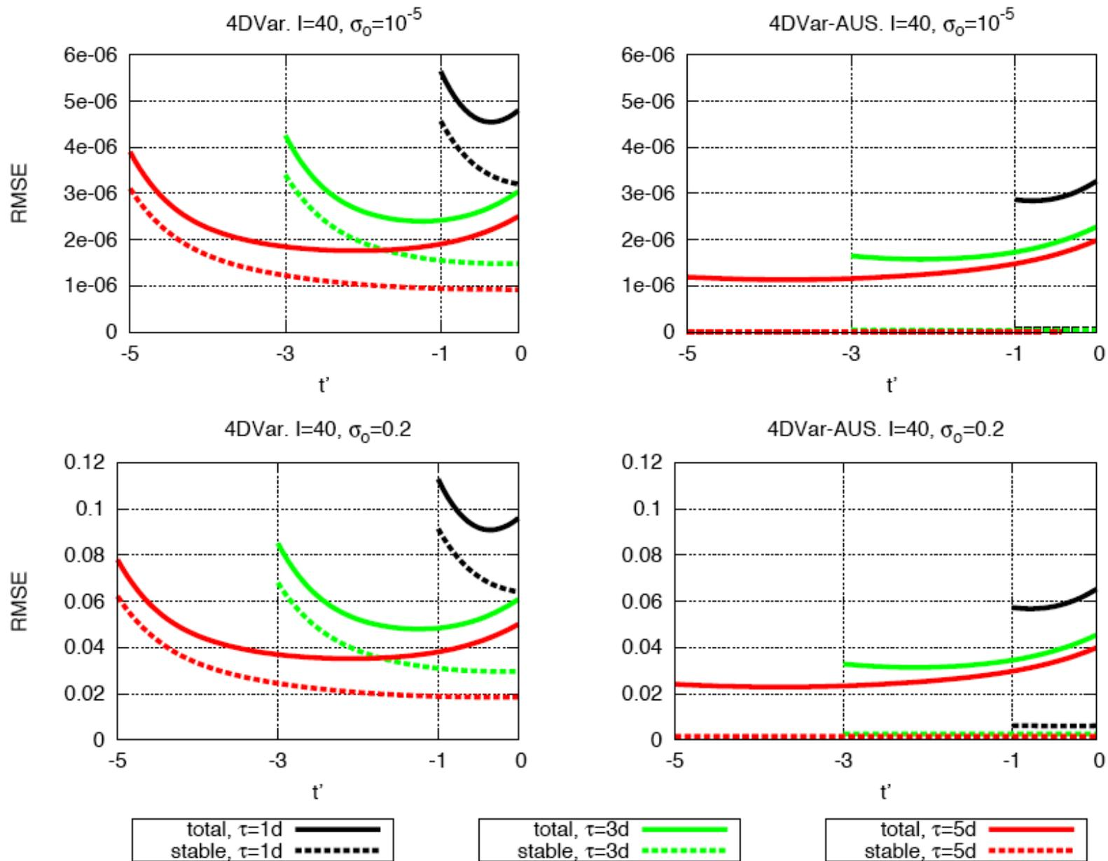
Figure 3. Time average RMS error within 1, 3, 5 days assimilation windows as a function of  $t' = t - \tau$ , with  $\sigma_0 = .2, 10^{-5}$  for the model configuration  $I = 40$ . Left panel: 4DVar. Right panel: 4DVar-AUS with  $N = 15$ . Solid lines refer to total assimilation error, dashed lines refer to the error component in the stable subspace  $e_{16}, \dots, e_{40}$ .
