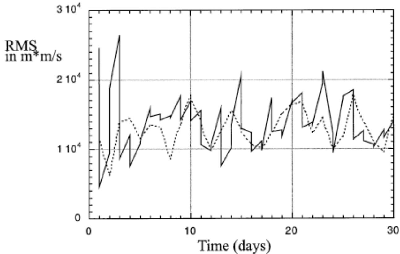
FIG. 12. Comparison of rms error ( $\text{m}^2 \text{s}^{-1}$ ) between ensemble mean and independent observations (dotted line) and the std dev in the ensemble (solid line). The excellent agreement shows that the SIRF is working correctly.
