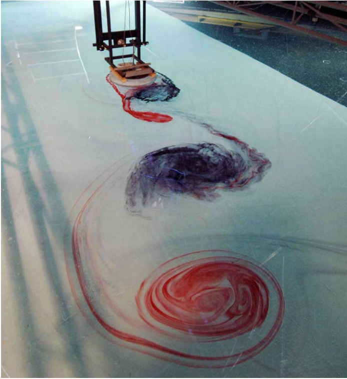
Figure 6. Dye visualisation of von Karman wake in a rotating shallow-water layer with \alpha \simeq 0.07 , Ro \simeq 2 and Re \simeq 20000 . Small-scale instability is visible in anticyclonic vortices (black dye), while cyclonic vortices (red dye) remain stable (Teinturier, Stegner, Viboud, Didelle and Ghil, 2006).
