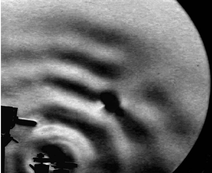
Figure 11. Optical altimetry visualisation of inertia-gravity waves (50 μm in amplitude) interacting with a localized vortices. The wave maker is on the bottom left, while the vortices appears in the center. Courtesy Y. Afanasiev.
