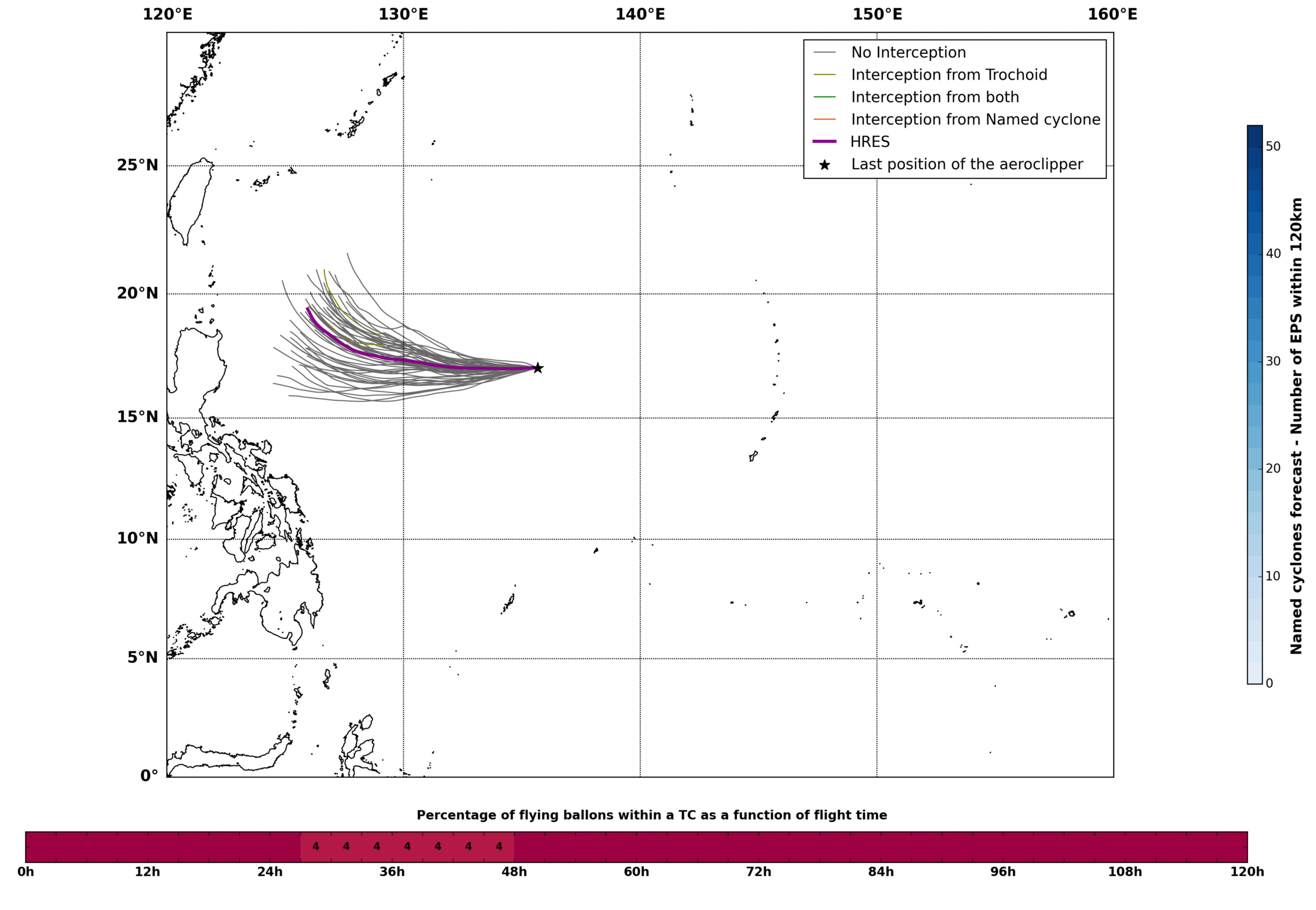
Aeroclipper CHL-PRL Grounding forecast from aeroclipper's position at 2022/05/09, 07h00 (UTC)
