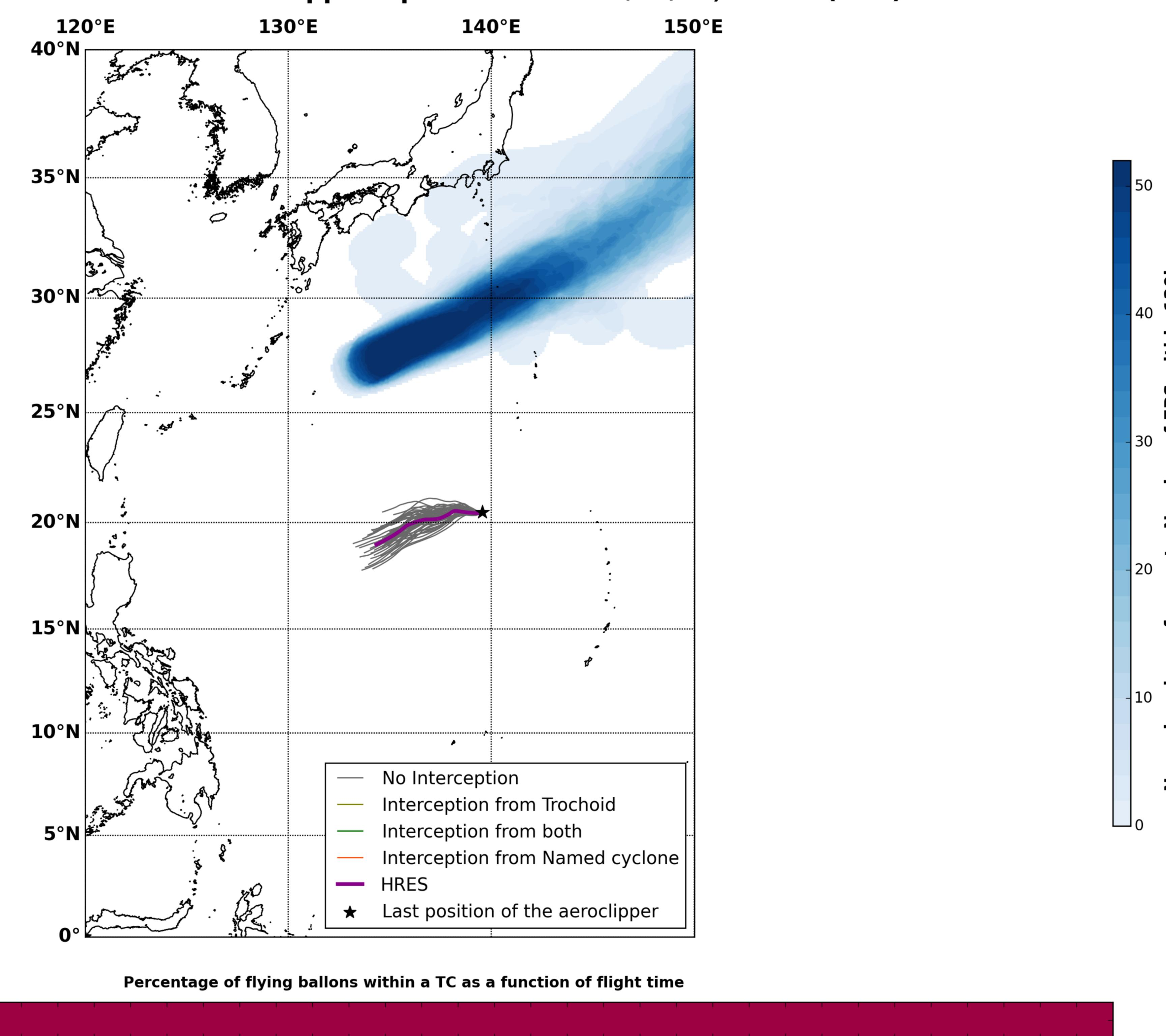
Aeroclipper DYL-BKA Grounding forecast from aeroclipper's position at 2022/09/29, 16h00 (UTC)
