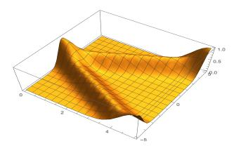
Solution in the domain -5 < x < 5, 0 < t < 5. Initial Gaussian perturbation propagates along a pair of characteristic lines with slopes  $\pm c$ . Graphics by Mathematica<sup>®</sup>
