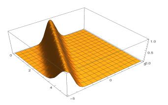
Solution in the domain -5 < x < 5, 0 < t < 5. Initial Gaussian perturbation propagates along a characteristic line with a slope *c*. Graphics by Mathematica<sup>®</sup>
